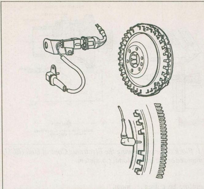
Fig. 6. Flywheel reluctor sensor. This comprises a magnet with a projecting pole piece and a reluctor disk on the flywheel.
