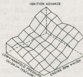
Fig. 8. Engine map using the programmed ignition system.
